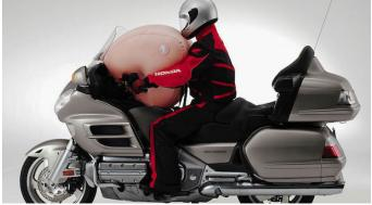
Figure 2 - Honda Goldwing equipped with an airbag
