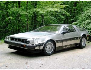
Figure 3- This DeLorean, also made out of stainless steel, will need an entirely new fender in order to be repaired
