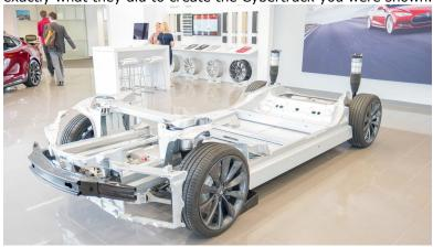
Figure 1 - Tesla Model S Skateboard chassis
