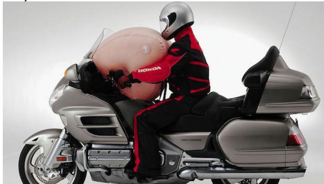
*Figure 2 - Honda Goldwing equipped with an airbag*
