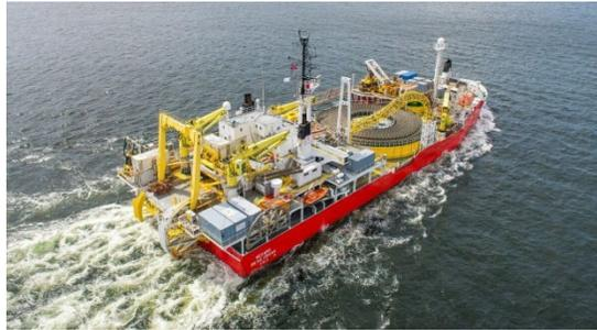
Figure 4 - The cable laying ship Nexans Skagerrak
