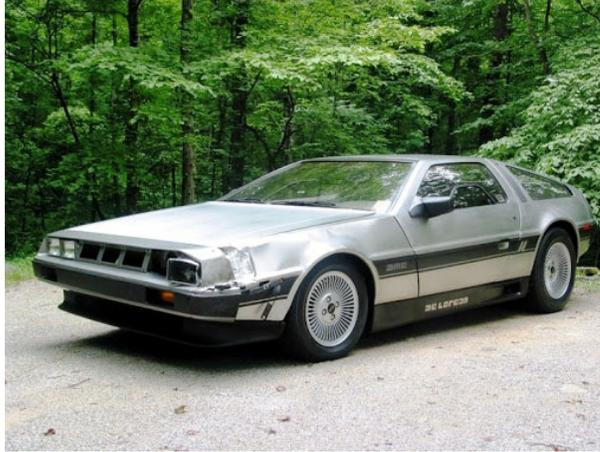
*Figure 3- This DeLorean, also made out of stainless steel, will need an entirely new fender in order to be repaired*
