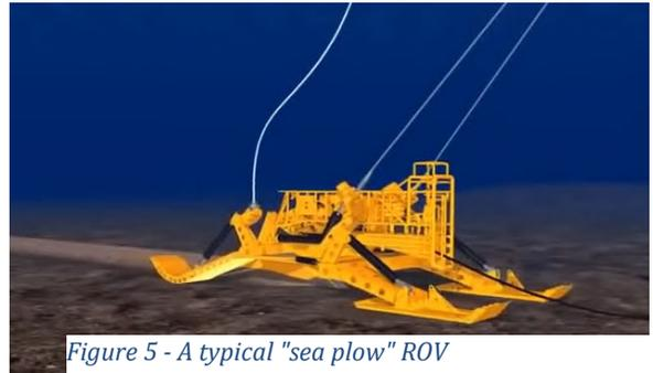
Figure 5 - A typical "sea plow" ROV
