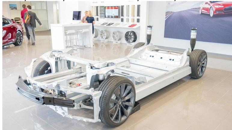
Figure 1 - Tesla Model S Skateboard chassis
