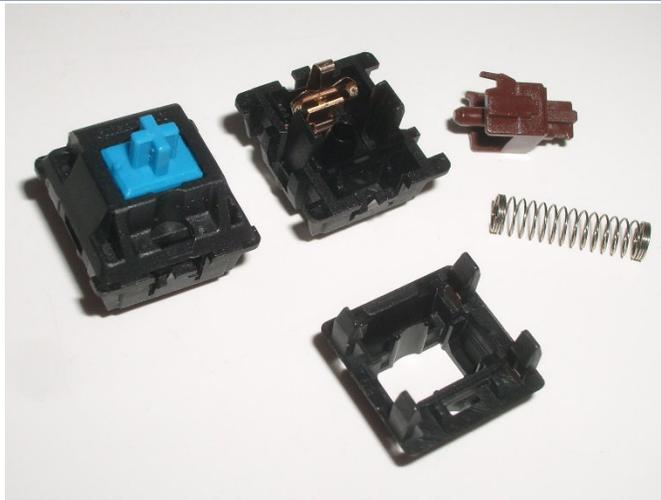
An assembled and disassembled mechanical switch. Left is MX Cherry Blue (clicky) and right is MX Cherry Brown (tactile).
